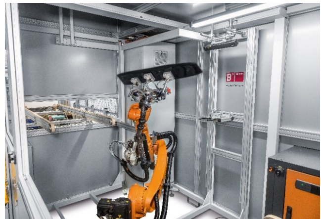
The robot then picks up the assembly and places it in the actual testing position. The second 3-D scanner displays the 3-D data for our specially developed virtual camera.
