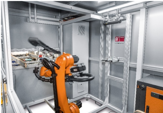
Absolutely flexible: The scanner transmits this information to a robot in a fraction of a second. This robot is thus able to pick up the respective assembly quickly and safely..
