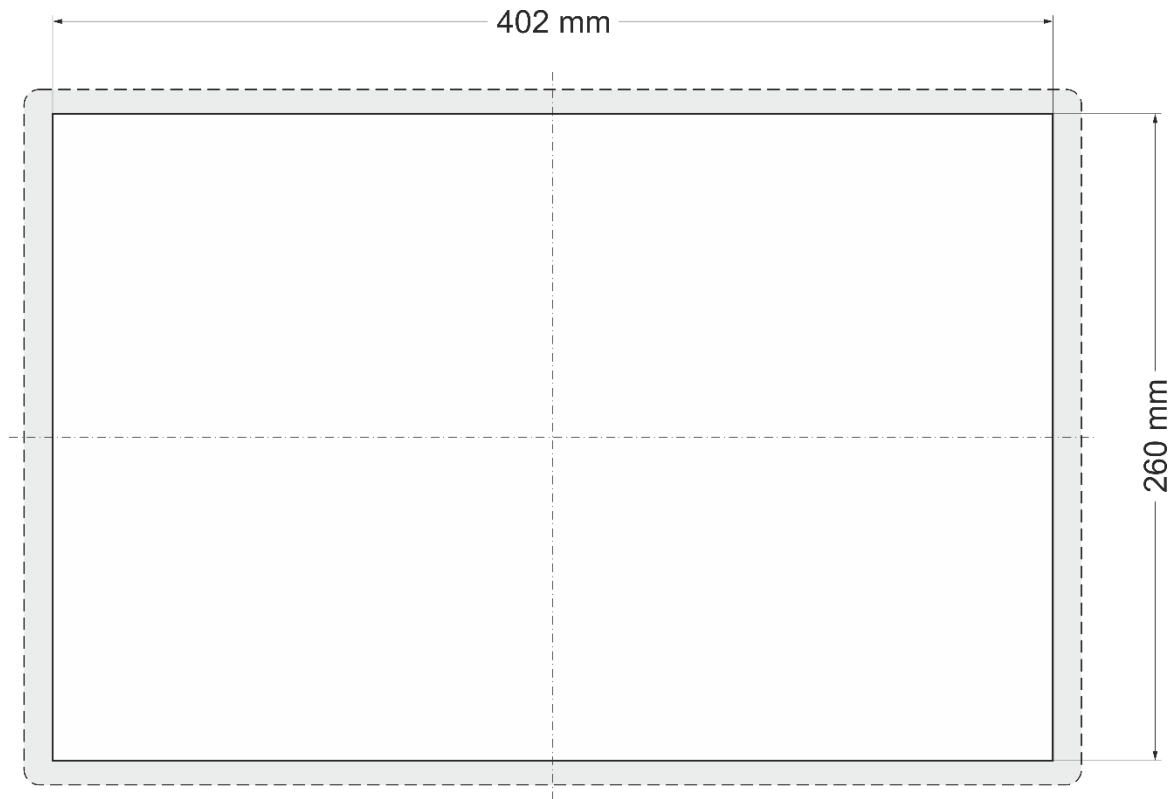
Fig. 13:DC-Pro 15 and ET-Pro 15 installation cut-out
