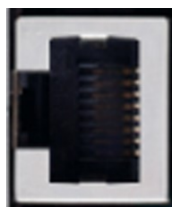
Fig. 41: CAN interface X7 (X12)
