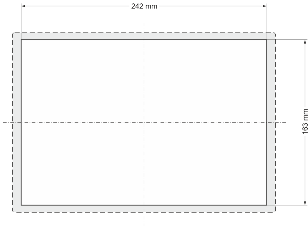
Fig. 5: Installation cut-out ET-Prime 10
